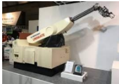
ABOVE: UNIMATE ROBOTIC ARM BY DEVOL
